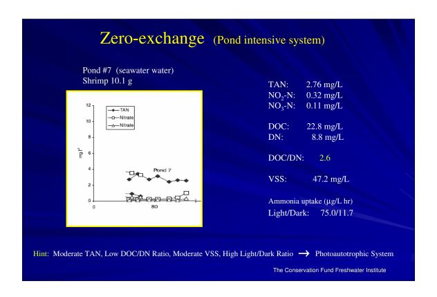
The high TAN concentrations and low nitrite and nitrate concentrations suggest that this pond has not generated sufficient AOB to begin the autotrophic process even with low C/N ratio. Light bottle/dark bottle ammonia uptake data indicates that TAN uptake by phytoplankton is the dominate pathway for TAN removal.
