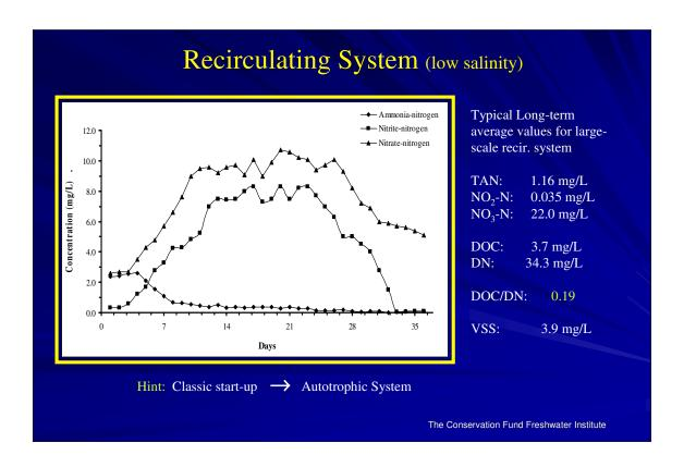
Water quality data for TAN (low), nitrite (moderate and falling) and nitrate (high) suggest a strong and robust autotrophic nitrification of TAN. Low C/N ratio would limit the heterotrophic bacteria growth.
