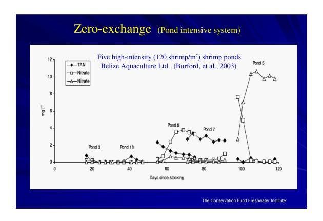
Water quality data from five research ponds over 3 week interval. Stocking density 120 shrimp/m<sup>2</sup>, grain based 21.9% and 35% protein feeds.
