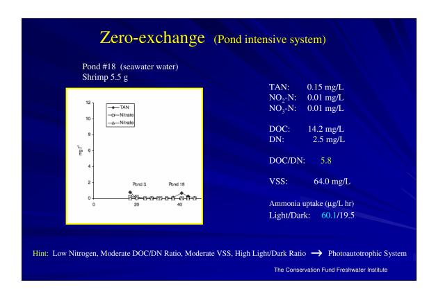
The high ammonia removal rate by the light bottle compared to dark bottle suggests a photoautotrophic system, which is supported by the low DOC/DN ratio. Also the pond was filled with fresh seawater, thus the low DOC compared to the previous pond filled with recirculated water. The moderate VSS concentration fits with the rapid growth and high yield of algae. The slight increase in TAN also is characteristic of the bloom and crash sequence seen in algae based systems.
